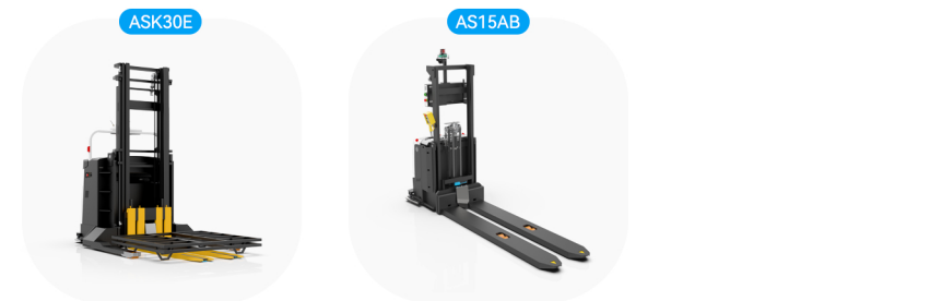
ASK30E: Quadruple forks, Rated load: 3000KG AS15AB: Extended fork storage, Rated load: 1500KG
