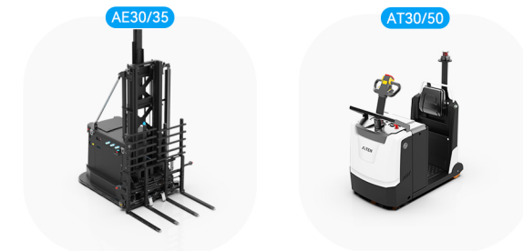
AE30/35: Quadruple forks, Rated load: 3000/3500KG AT30/50: Towing robot, Rated load: 3000/5000KG
